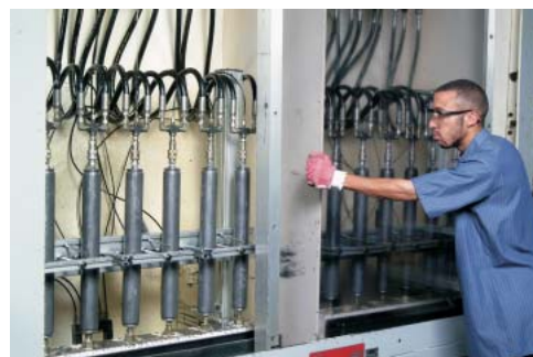
Every accumulator is cycle tested prior to shipment.
